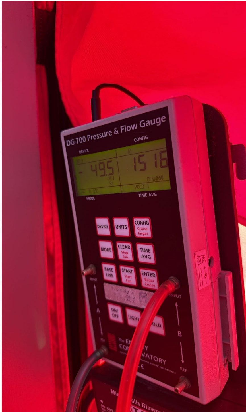
Figure 11-4: Air Infiltration Project- High CFM50 Post Air Infiltration Test Result
