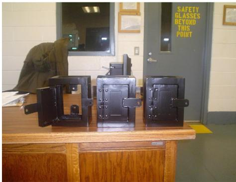
EARU CTE designed and fabricated three secure metal boxes to be used to store emergency rescue medical supplies.
