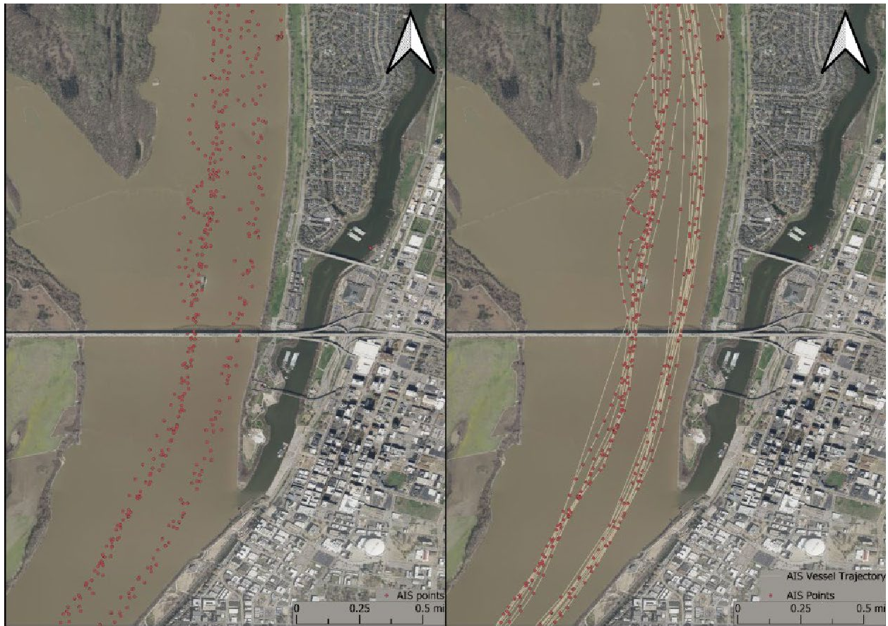
Figure 18. From raw data to vessel tracks at the I-40 bridge. The scattered points on the left are processed to create the clear vessel trajectories shown on the right
