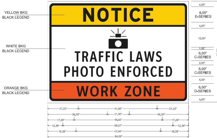
WZ-1 (INTERSTATE) SIGN
