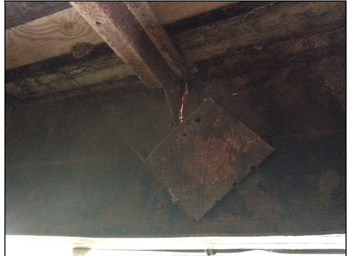
Crack on main beam car 1
