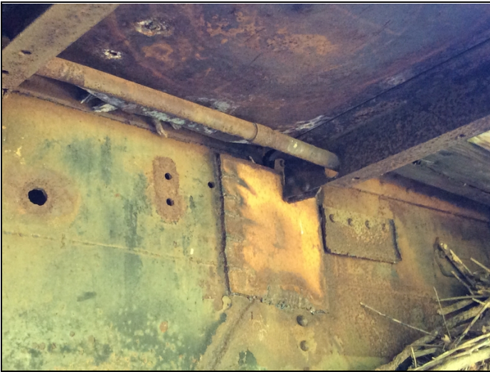
Crack outside of main sill. Plate welded over crack crack still visible above plate
