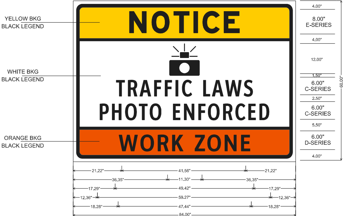
WZ-1 (INTERSTATE) SIGN
