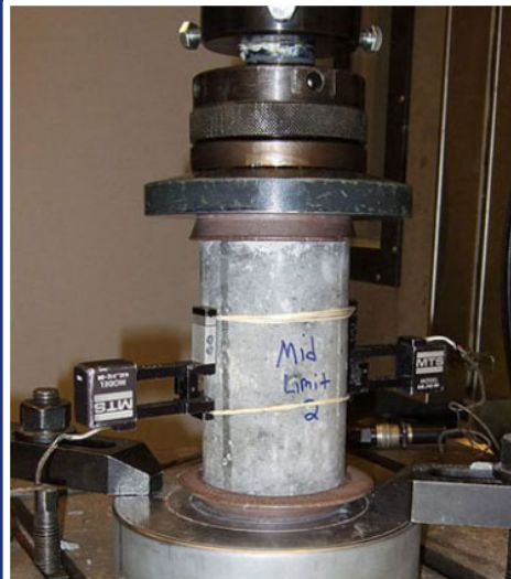
Concrete strength test
