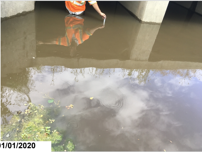
The inlet end of barrel #3 has a 2' deep scour hole.
