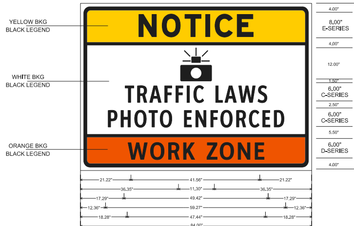
WZ-1 (INTERSTATE) SIGN
