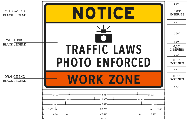
WZ-1 (INTERSTATE) SIGN
