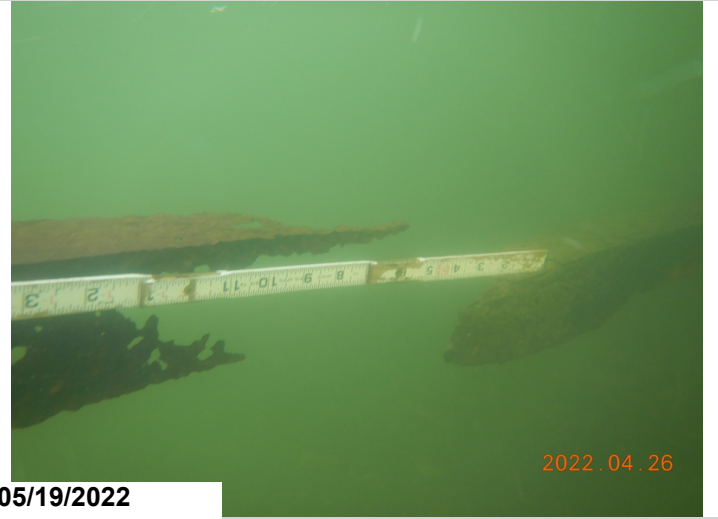
BENTS 2 & 3, CORROSION ON CROSS BRACING WITH UP TO 100% SECTION LOSS
