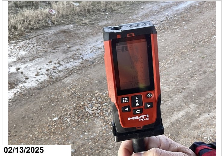
11' 4" verification noted at girder 1, right.
