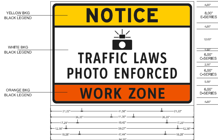
WZ-1 (INTERSTATE) SIGN
