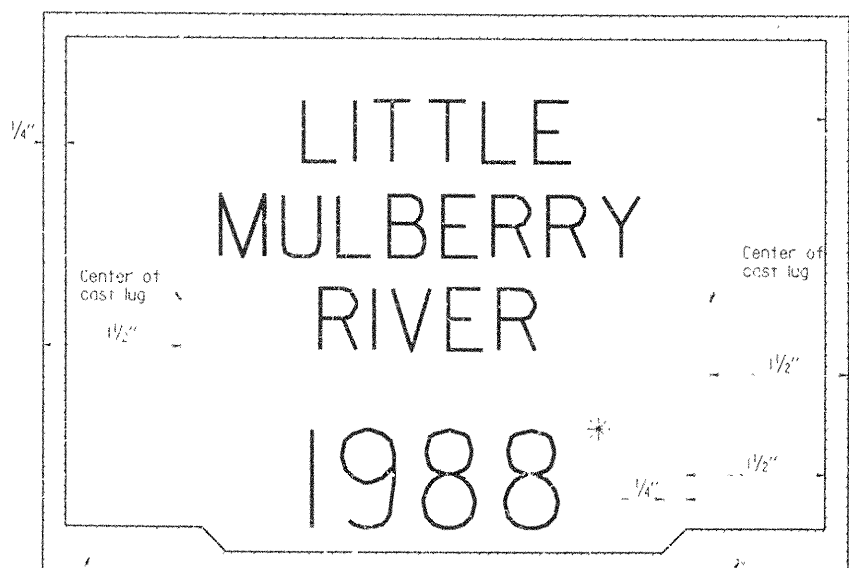
TYPICAL BRIDGE NAME PLATE-STYLE 2-FULL SIZE STREAM CROSSINGS
