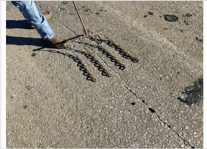
Span 2 Left approx 8ft delaminated area
