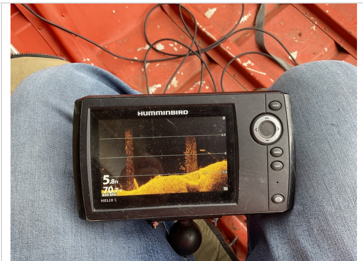
Bent #2 no apparent scour problems.
