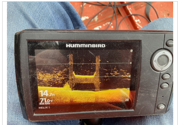
Bent #3 no apparent scour problems.
