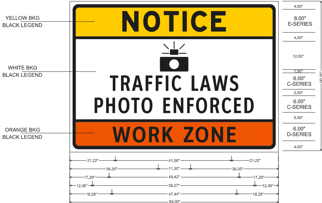
WZ-1 (INTERSTATE) SIGN
