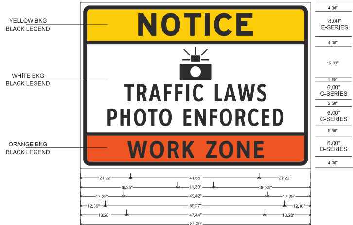
WZ-1 (INTERSTATE) SIGN
