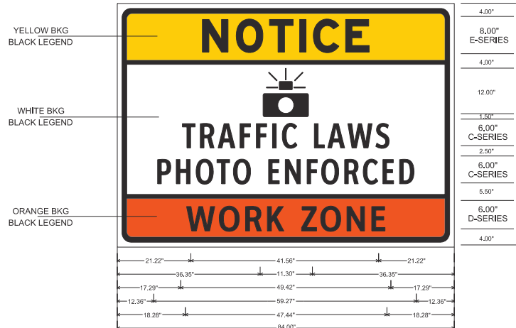
WZ-1 (INTERSTATE) SIGN
