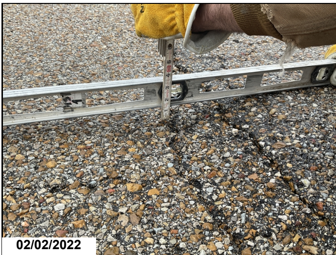
Abutment #1 right lane approach roadway has settled one inch
