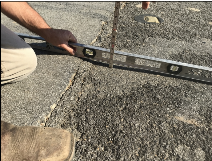
Abutment #1 approach roadway settlement.
