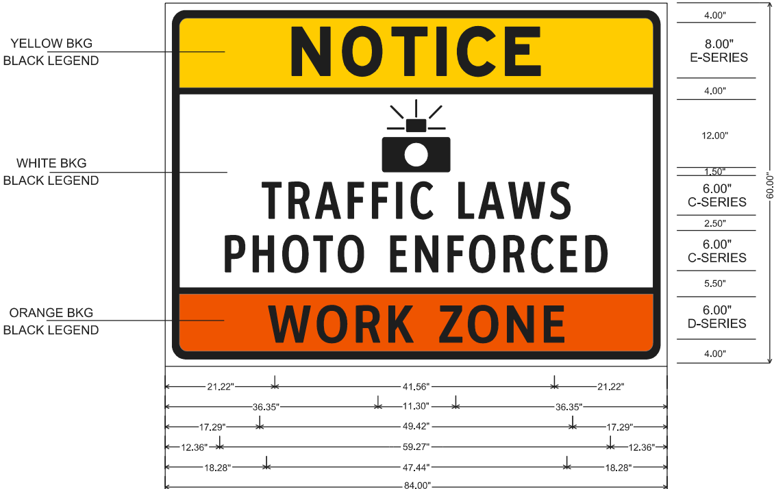
WZ-1 (INTERSTATE) SIGN
