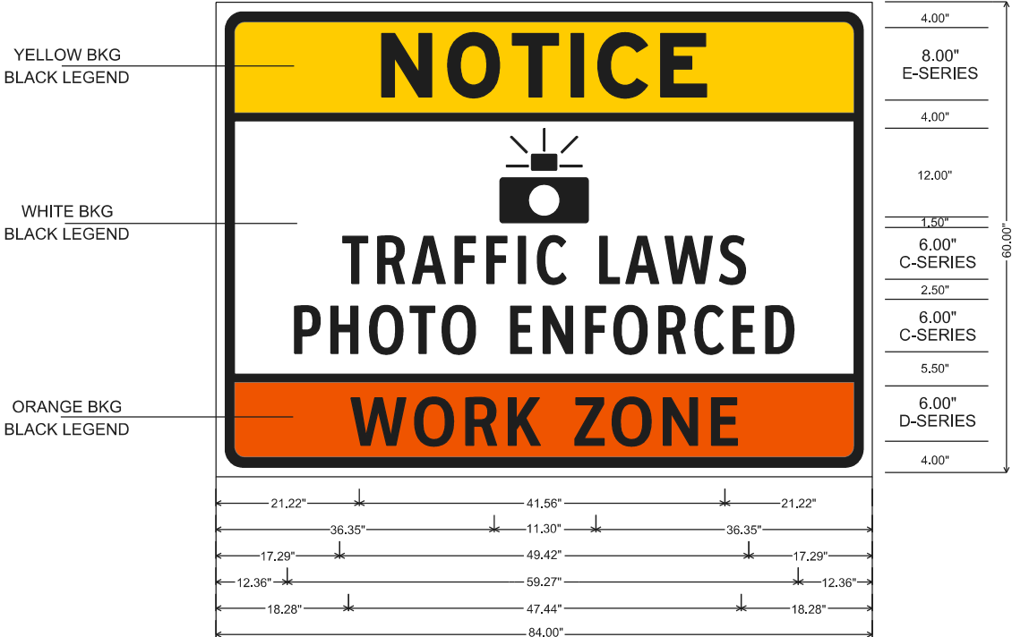
WZ-1 (INTERSTATE) SIGN
