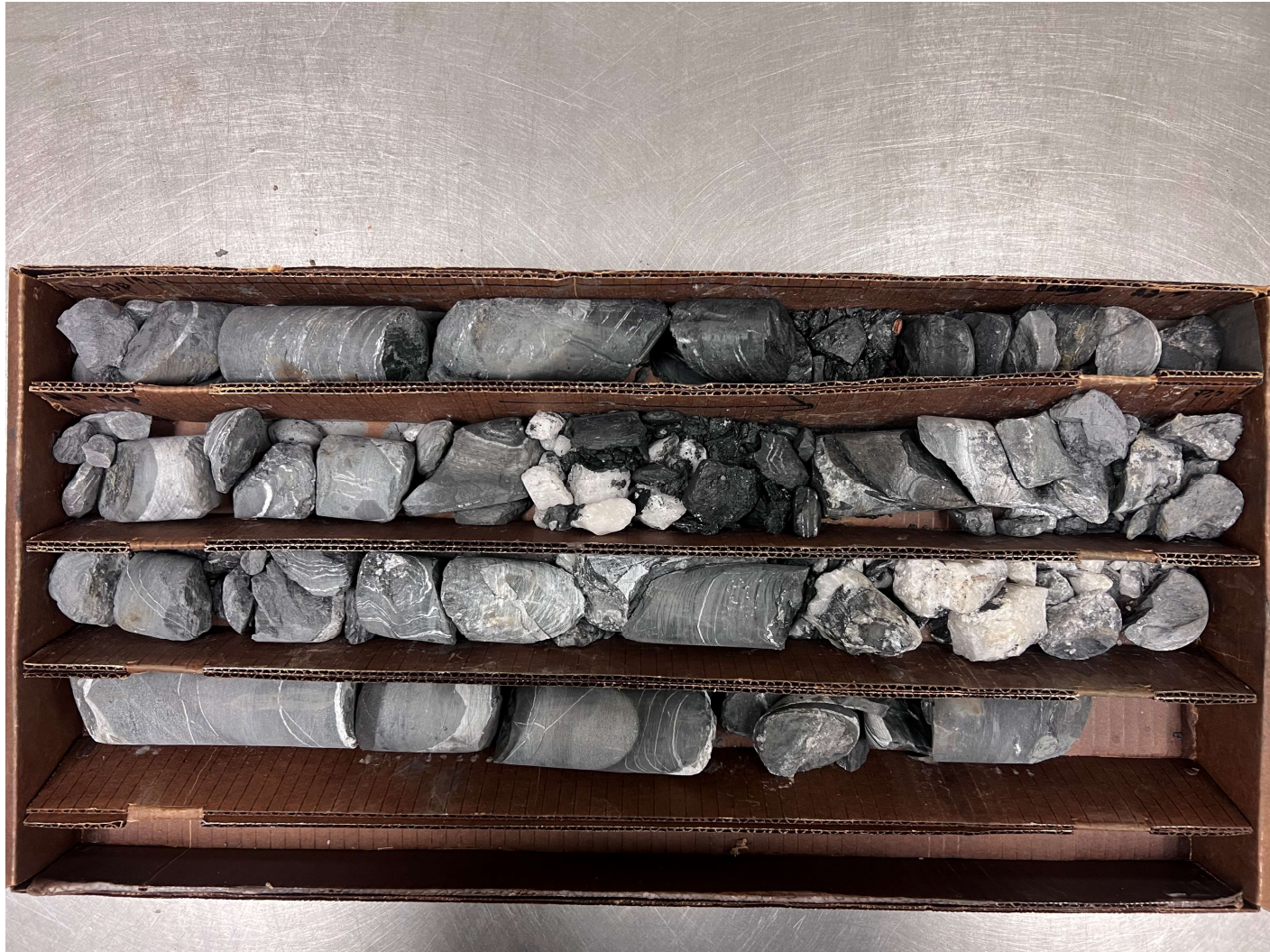
Station and Offset, ft: Sta. 105+14, 13 feet Right of Construction Centerline (Boring 2) Depth, ft: 19.2 – 32.7
