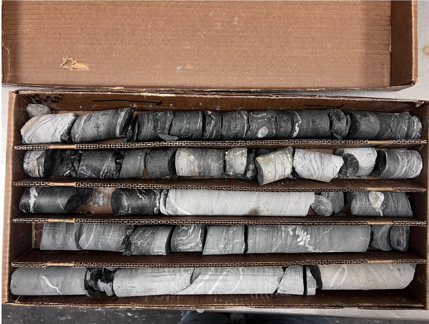
Station and Offset, ft: Sta. 103+95, 13 feet Right of Construction Centerline (Boring 1) Depth, ft: 28.7 – 38.7
