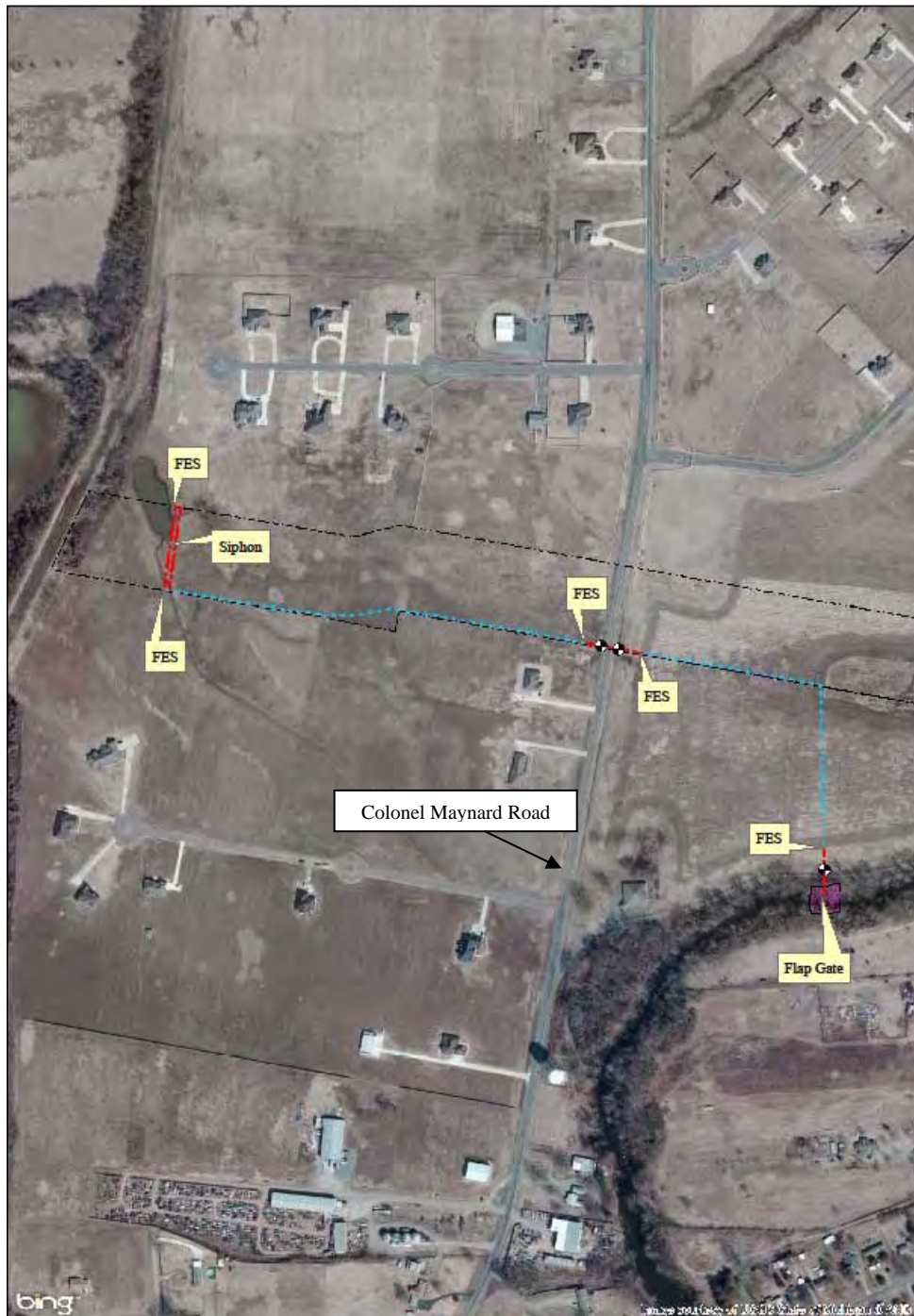
Figure 3. The blue line represents the proposed drainage route for the stormwater diversion from a low area near Canal 1000 to Scott Bayou near Scott, Arkansas. FES refers to “Flaired End Sections” at the entrance and exit of culverts.
