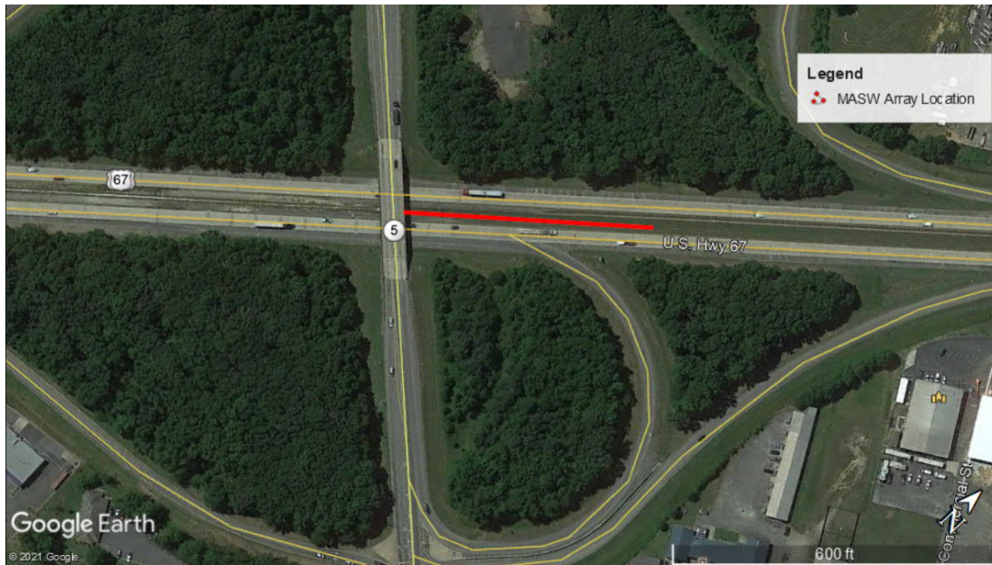
Figure 4. Location of MASW Array – U.S. 67 Over Two Prairie Creek
