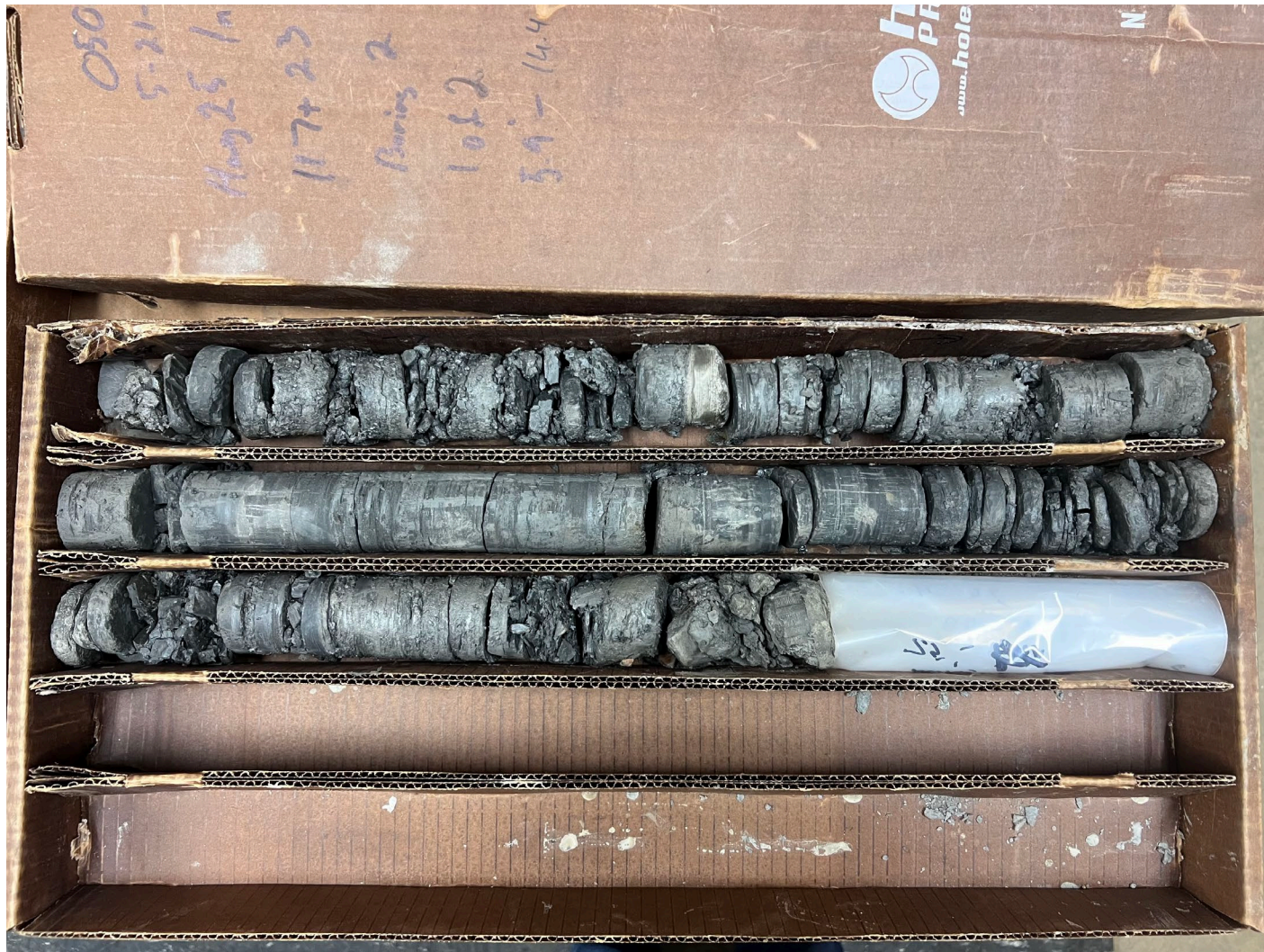
Station 117+23, Construction Centerline (Boring 2) Depth, ft: 5.9 – 14.4
