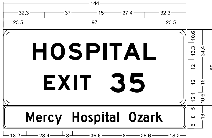
ML40-35-9EB; 6.0" Radius, 2.0" Border, White on Blue; "HOSPITAL", E Mod 2K; "EXIT", E Mod 2K; "35", E Mod 2K; 3.0" Radius, 1.0" Border, White on Blue; "Mercy Hospital Ozark", D 2K;
