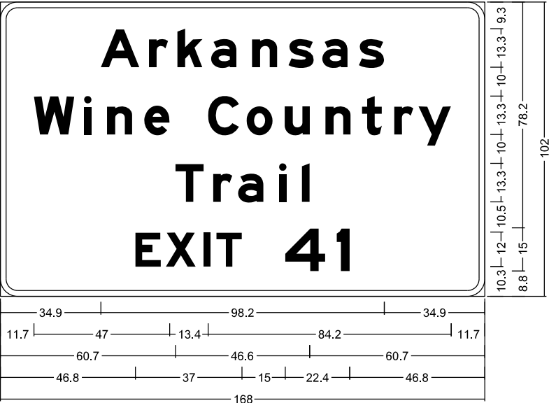
ML40-41-5WB; 6.0" Radius, 2.0" Border, White on Brown; "Arkansas", E Mod 2K; "Wine Country", E Mod 2K; "Trail", E Mod 2K; "EXIT", E Mod 2K; "41", E Mod 2K;
