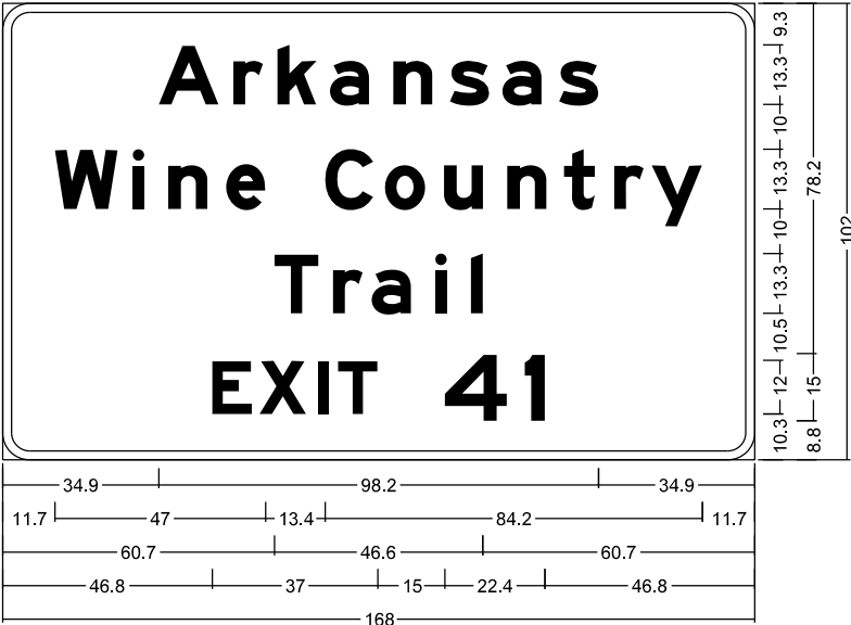
ML40-41-4EB; 6.0" Radius, 2.0" Border, White on Brown; "Arkansas", E Mod 2K; "Wine Country", E Mod 2K; "Trail", E Mod 2K; "EXIT", E Mod 2K; "41", E Mod 2K;
