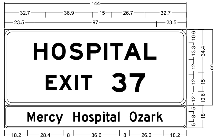
ML40-37-5WB; 6.0" Radius, 2.0" Border, White on Blue; "HOSPITAL", E Mod 2K; "EXIT", E Mod 2K; "37", E Mod 2K; 3.0" Radius, 1.0" Border, White on Blue; "Mercy Hospital Ozark", D 2K;
