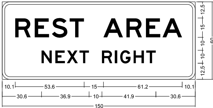
ML40-RA-2EB; 6.0" Radius, 2.0" Border, White on Blue; "REST AREA", E 2K; "NEXT RIGHT", E 2K;
