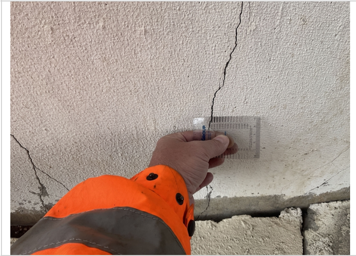
Bent # 2 Column #3 with 0.060" vertical cracks.
