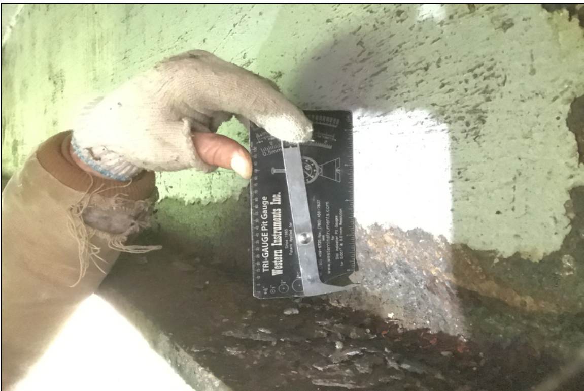
Span # 6, beam 1 over abutment 2-3/16" section loss to base of web.
