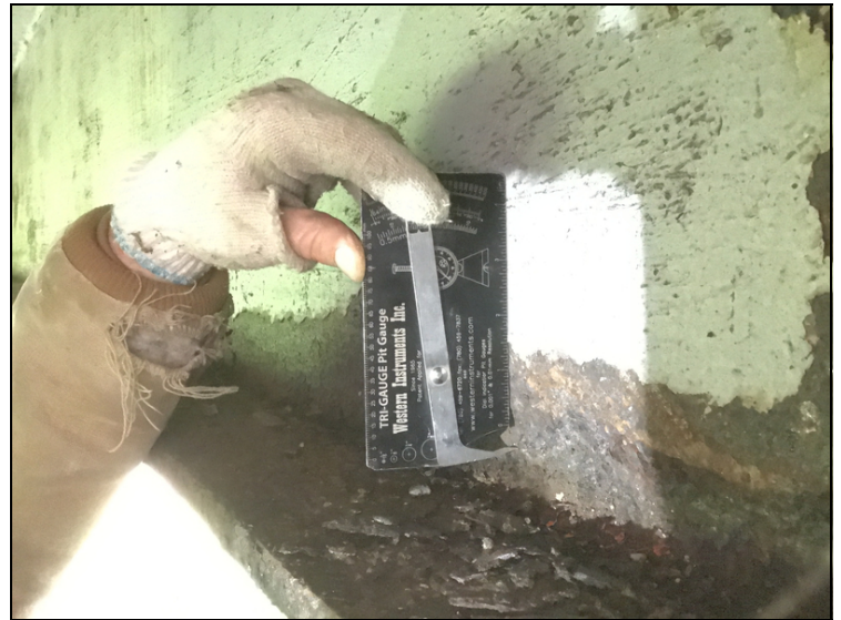
Span # 6, beam 1 over abutment 2-3/16" section loss to base of web.
