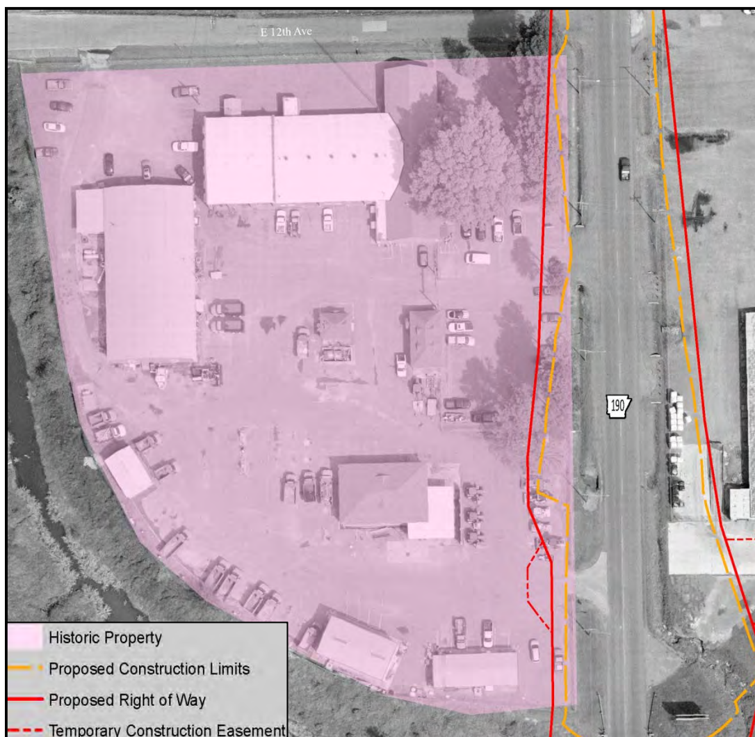
Figure 5. Proposed ROW to be acquired from the State Highway Department District 2 Complex
