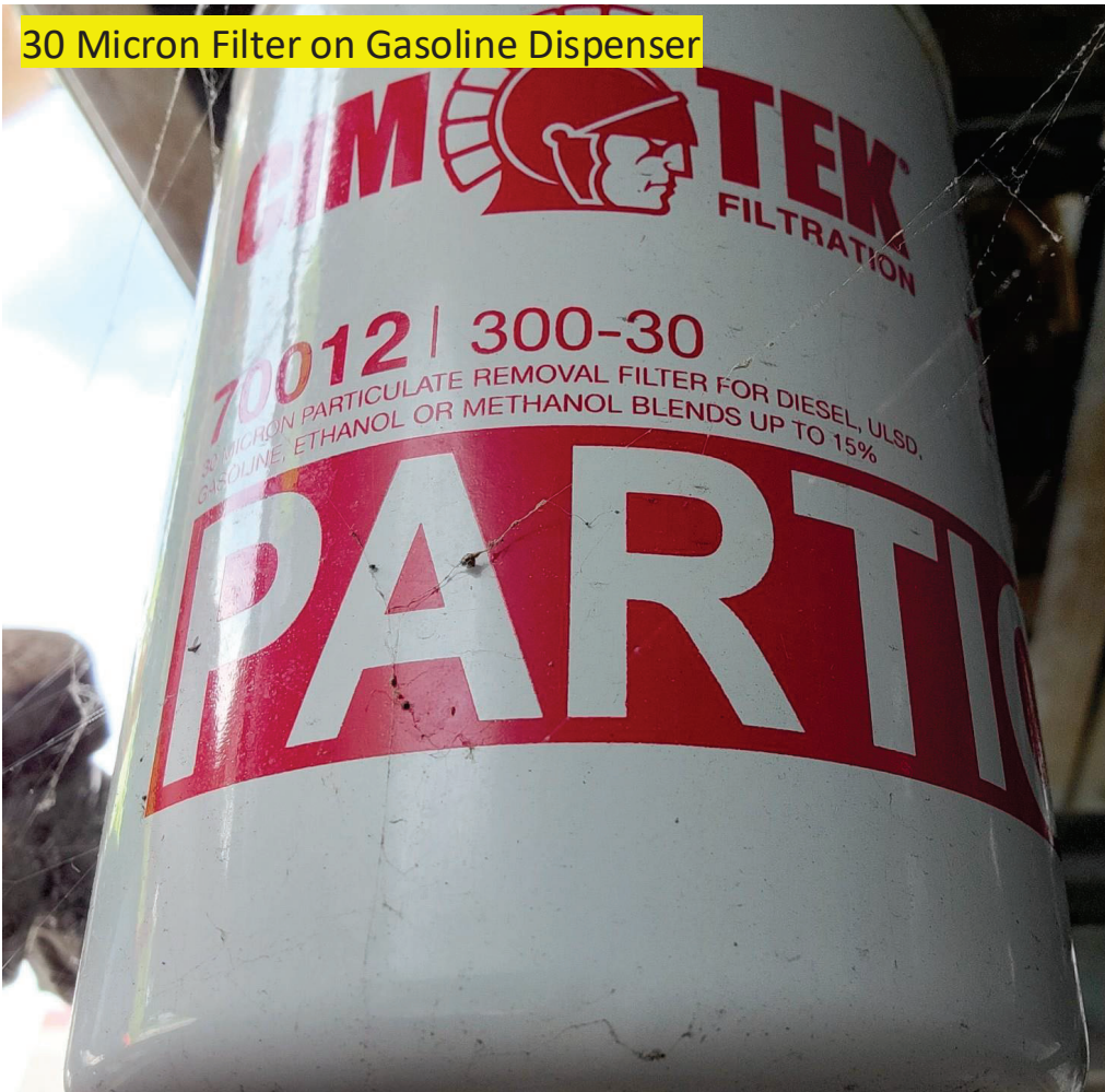
Only up to 10-micron pore-sized filters allowed on gasoline dispensers
